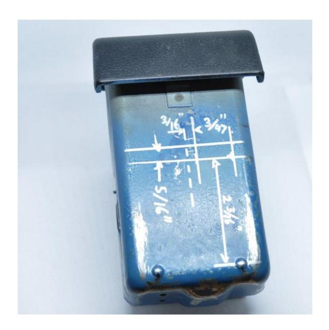
4 Drill a ¼" (6mm) hole for the wire exit hole at the back of the tray. Somewhere close to the white circle is ideal.
