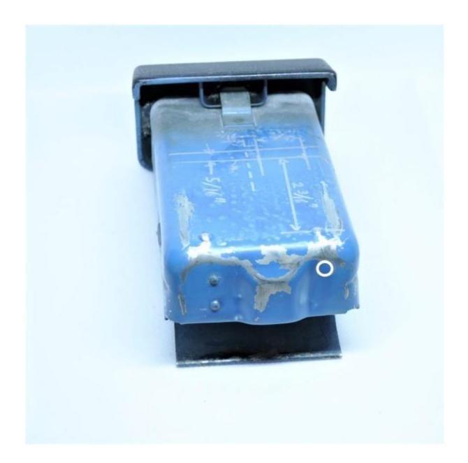
Drill another wire exit hole in the ashtray housing from under the hood approximately inline with the ashtray hole, remove any sharp edges with a larger drill, countersink or file. The wire needs to pass through both holes in a straight line for smooth opening and closing.
