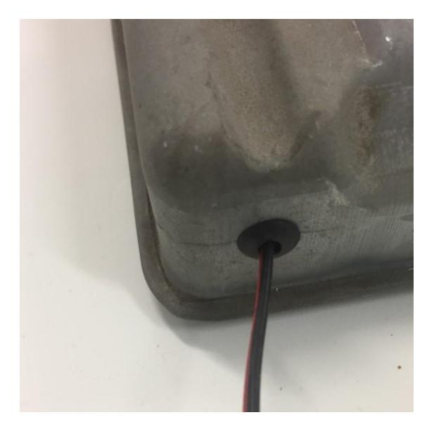
6 Hold the charger firmly in the desired position to the tray and screw in the self tapping screws. We do not recommend drilling pilot holes in the charger as it's easy to go too deep and into the circuitry causing damage. You can use a battery screwdriver but go slowly.
