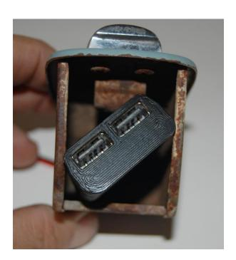
Hold the charger tight against the face you just drilled and as deep in the tray as it will go. It needs to sit deep to clear the retaining latch in the housing.
