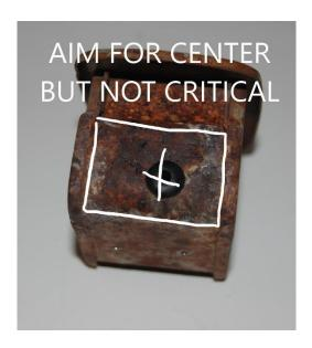
4 Drill a 1/4" hole for the second grommet in the ashtray housing. Position close to the first. Install grommet the same way then reinstall surround.
