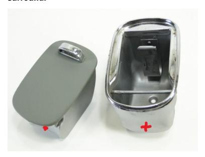
Drill two holes as per the drawing below. Positions are approximate as the screws are self tapping into solid 3D printed housing. Remove the burrs from inside with the end of a larger drill or file.
