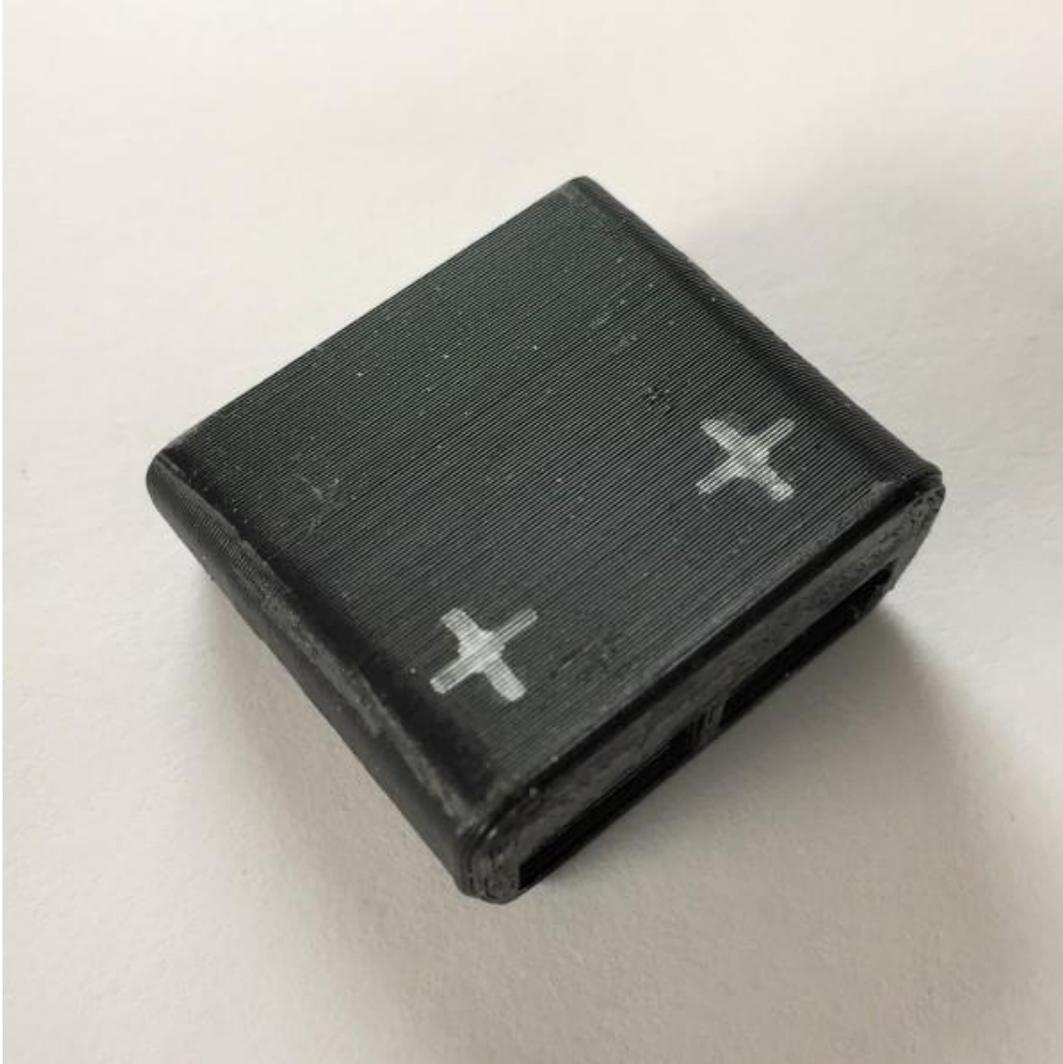
4. Mark your hole positions on the underside of the tray so they will so the screws will penetrate approximately where the marks are on the charger. With the charger removed, drill the ashtray 3/32" or 2.5mm and remove the burrs from inside with the end of a larger drill or file.
