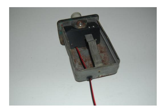
5 Connect your wires with your preferred method (a soldered joint is best). This unit works with both 6V and 12V systems.
