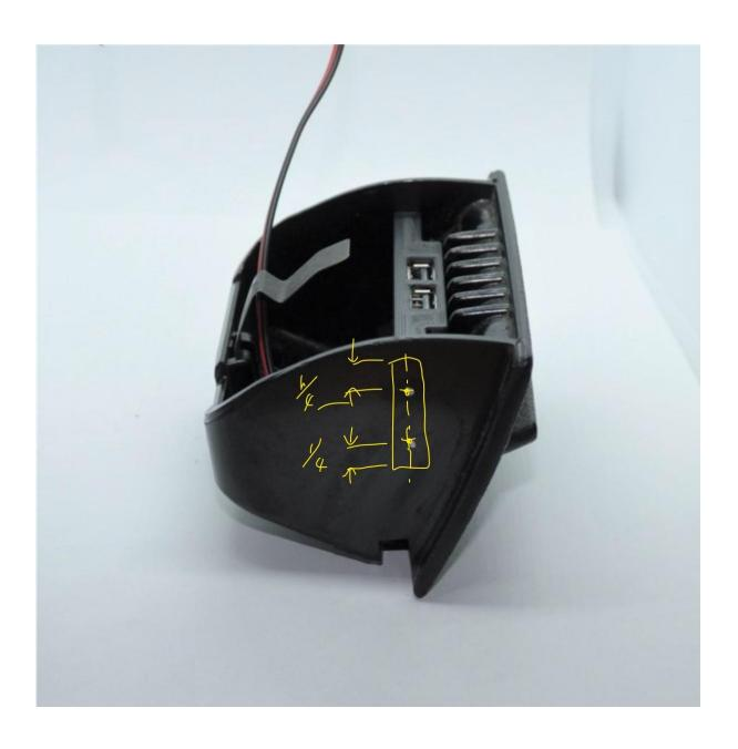
Drill a ¼" (6mm) hole for the wire exit hole at the back of the tray. Location isn't critical but the layout below works well. Drill carefully as this material is quite brittle.
