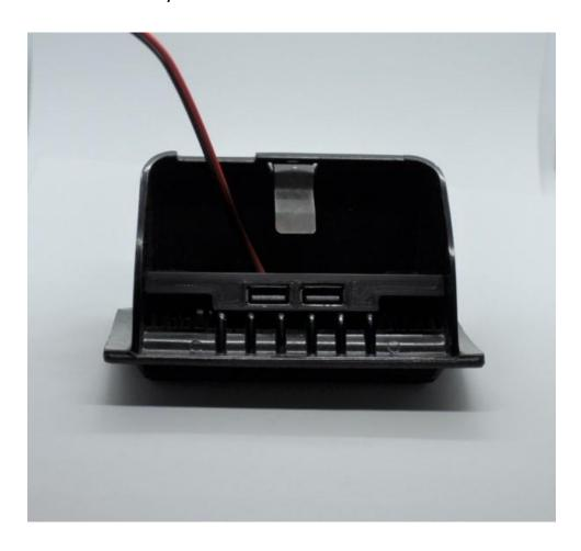
On the sides of the tray lay out the hole positions as shown. Vertically on the centerline of the charger face and  $\frac{1}{4}$ " (6mm) from each end.
