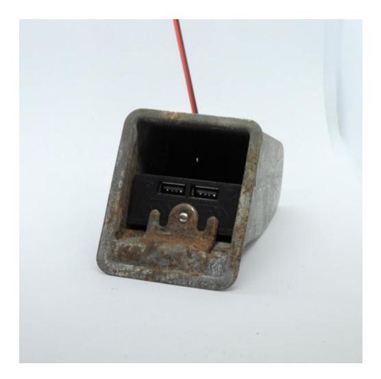
5 Connect your wires with your preferred method (a soldered joint is best, but crimp terminals will work.) Leave some slack to allow for the opening and closing of the ashtray.
