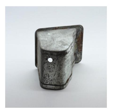
3 Remove any sharp edges on the hole with a deburring tool or larger drill bit. Insert the supplied grommet. (Softening it in hot water will make it easier.)
