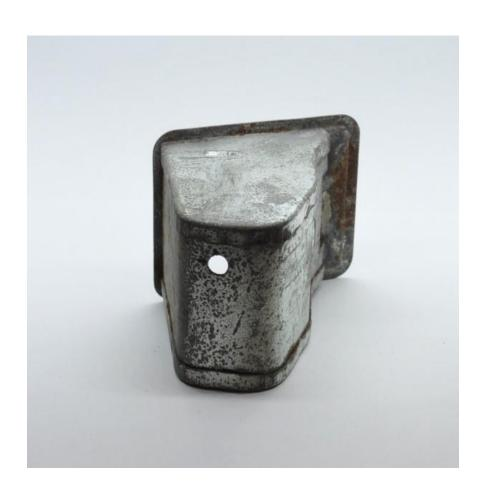
Remove any sharp edges on the hole with a deburring tool or larger drill bit. Insert the supplied grommet. (Softening it in hot water will make it easier.)
