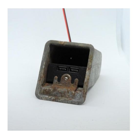
Connect your wires with your preferred method (a soldered joint is best, but crimp terminals will work.) Leave some slack to allow for the opening and closing of the ashtray.
