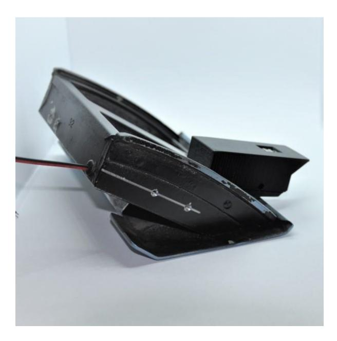
7 Hold the charger firmly in the final position to the tray and screw in the self tapping screws. We do not recommend drilling pilot holes in the charger as it's easy to go too deep and into the circuitry causing damage. A regular screwdriver with some pressure works best. You can use a battery screwdriver but go slowly.
