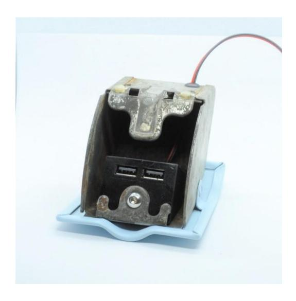
5 Connect your wires with your preferred method (a soldered joint is best) but a crimped connection will be adequate.
