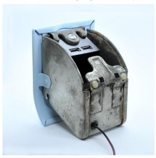
Remove the socket hex screw from the charger. Poke the wire through the hole, slide the grommet over the wire and insert the grommet in the hole. Warming the grommet in hot water will soften it for an easier install. Position the charger as shown below and secure with the USB ports towards the back of the ashtray and screw just tight enough to stop it moving, but not too tight.
