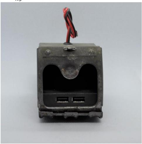
On the side of the ashtray lay out the two hole positions as shown below by the cross marks. They don't need to be exact as you will be screwing into solid plastic but within 1/16" (2mm) or so. Lay out the two holes 1/8" (3mm) from the edge of the return on the ribbed panel and 3/8" (10mm) and 1 1/8"(28mm) from the edge of the overlapping seam of the ashtray. Drill 3/32" (2.5mm) in those two spots and countersink.
