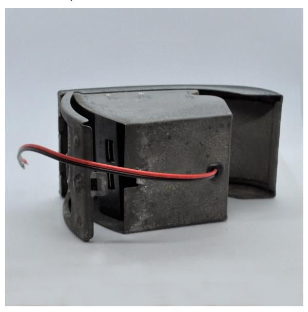
Re close the top of the ashtray. Hold the charger firmly in its final position, tight to the top and front of the ashtray and screw in the self tapping screws. We do not recommend drilling pilot holes in the charger as it's easy to go too deep and into the circuitry causing damage. You can use a battery screwdriver but go slowly. Ensure the screw heads are flush so they don't catch the dashboard during operation.
