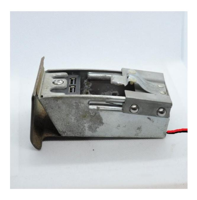
Prepare your power and ground wires behind the dash. Be sure to allow enough length to allow for the opening and closing of the ashtray.
