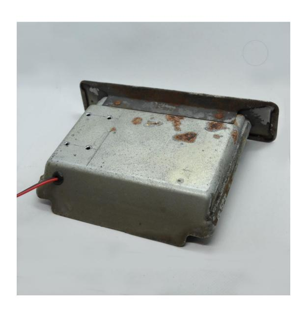
Hold the charger firmly in this position and screw in the four self tapping screws into the charger. Usually, no drilling of the charger is necessary. A manual screwdriver is best with firm pressure applied. If you do choose to use a drill or power driver, be very careful not to drill/screw too deep as the circuit board can be damaged.
