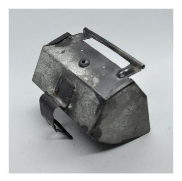
5 Thread the wire through the ashtray hole as in image below and then reattach the fascia etc. On the ashtray used in the photos, the original screws were just long enough to reuse. If yours aren't, replace with 1/8" longer ones.
