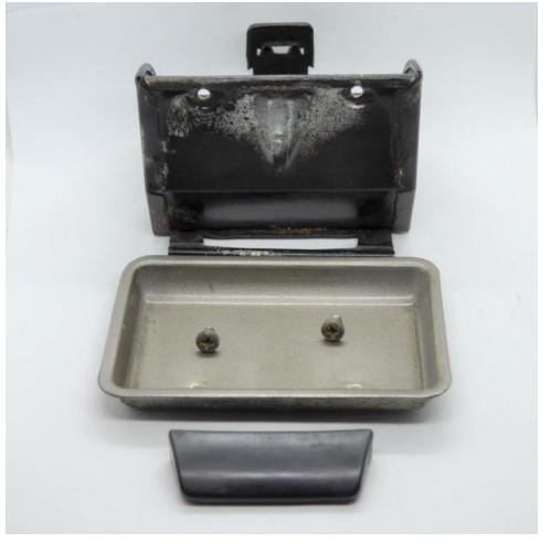
Drill a ¼" (6.5mm) hole for the wire exit hole at the bottom of the back of the tray. Check for obstructions where the wire will exit prior to drilling.
