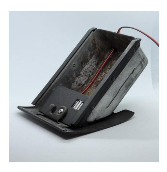
Insert your ashtray into the dash (not shown) with the power wire going in first. Disconnect the battery, then connect your wires with your preferred method. Red to power and black to ground. A soldered joint is best, but a crimped connection will be adequate. Remember to leave some slack in the wire to allow for the movement of the ashtray.
