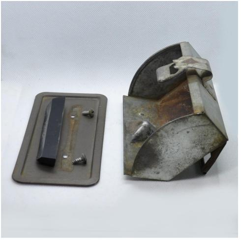
3 Drill a ¼" (6.5mm) hole for the wire exit hole in the corner of the back of the tray. Check for obstructions and a clear path where the wire will exit prior to drilling. The left hand corner (from the drivers seat) as shown below should works well but double check if that location works for your vehicle before drilling.
