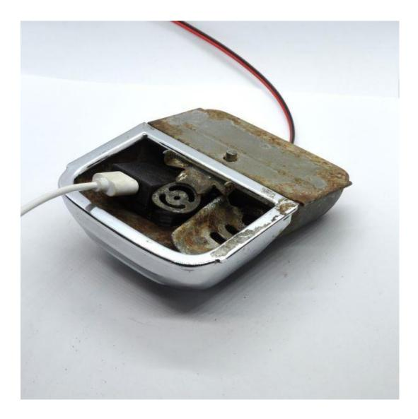
8 Prepare your power and ground wire under the dash. Reinstall the ashtray, connect your power to red and ground to black. This unit works with both 6V and 12V systems.
