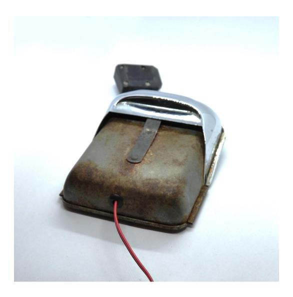
7 Position the charger with the top edge in line with the edge of the disc in the center of the stubber as per the yellow line in the image below. Lateral location is as close as can be to the stubber without it touching. The stubber needs clearance, so as to be able to pressed up and down, as it is also the release mechanism for ashtray removal. Firmly hold the charger in the desired position and screw in the three self tapping screws.
